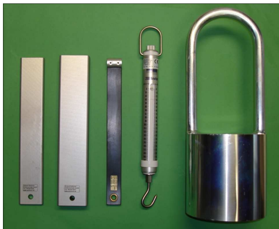
Measurement rod 1 (10 mm x 50 mm) Measurement rod 2 (30 mm x 60 mm) Measurement rod 3 Spring Balance Measurement rod 4
