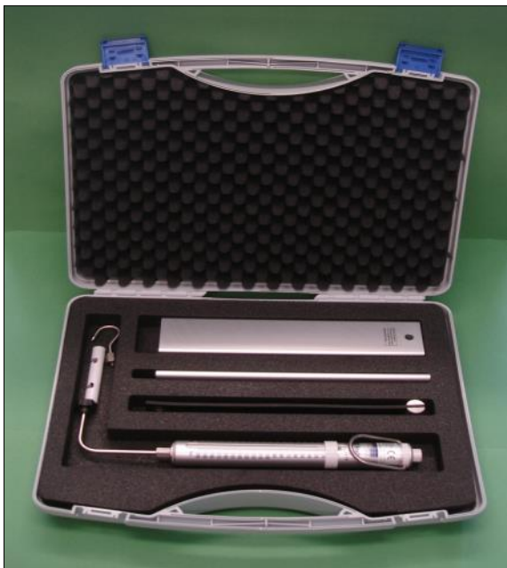
Case for measurement rods 1 to 3 with spring balance
