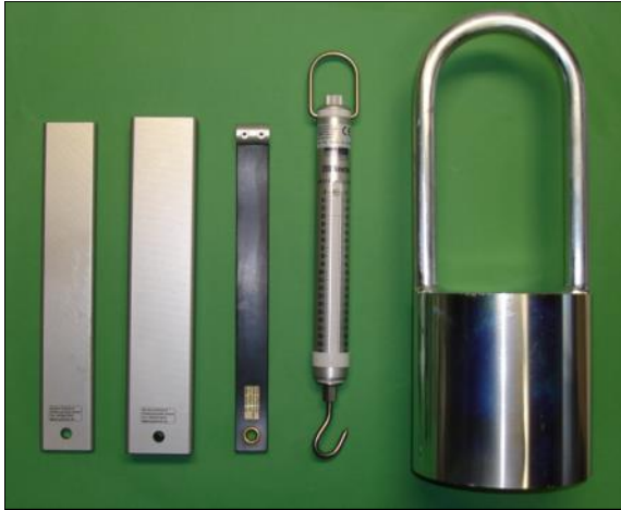
Measurement rod 1 (10 mm x 50 mm x 300mm) Measurement rod 2 (30 mm x 60 mm x 300mm) Measurement rod 3 Spring Balance Measurement rod 4
